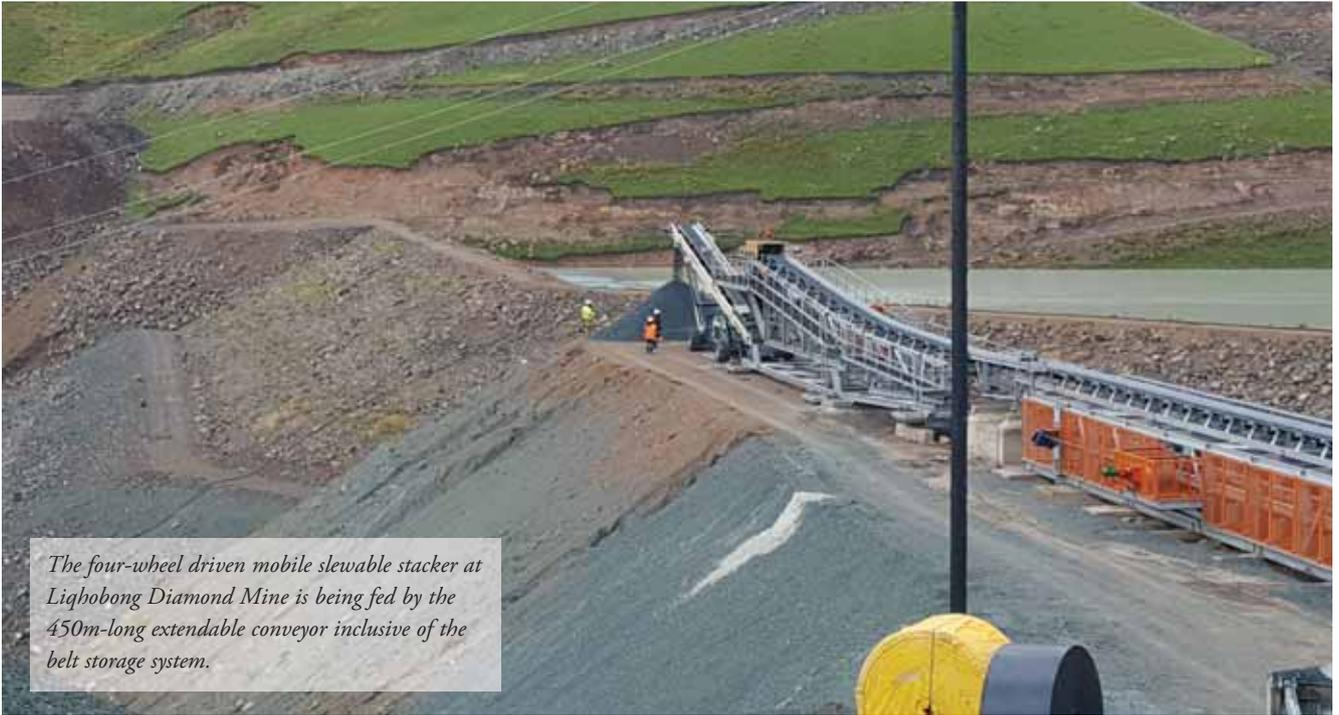
*The four-wheel driven mobile slewable stacker at Lihobong Diamond Mine is being fed by the 450m-long extendable conveyor inclusive of the belt storage system.*
