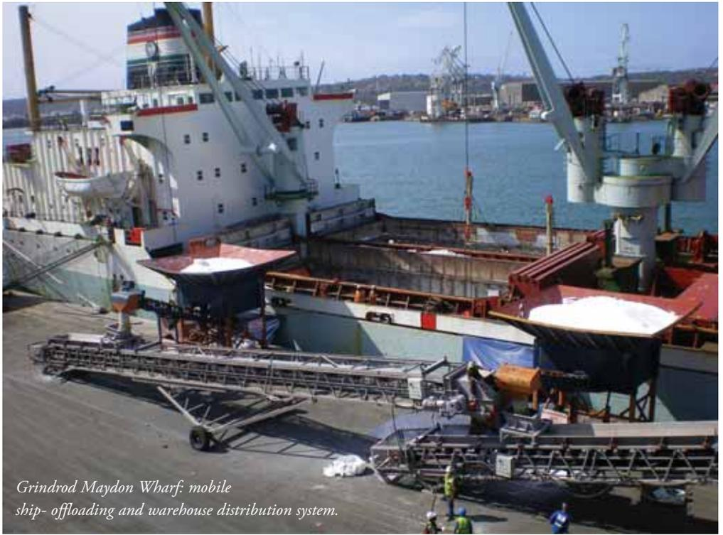
*Grindrod Maydon Wharf: mobile ship-offloading and warehouse distribution system.*
