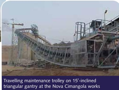
Travelling maintenance trolley on 15°-inclined triangular gantry at the Nova Cimangola works
