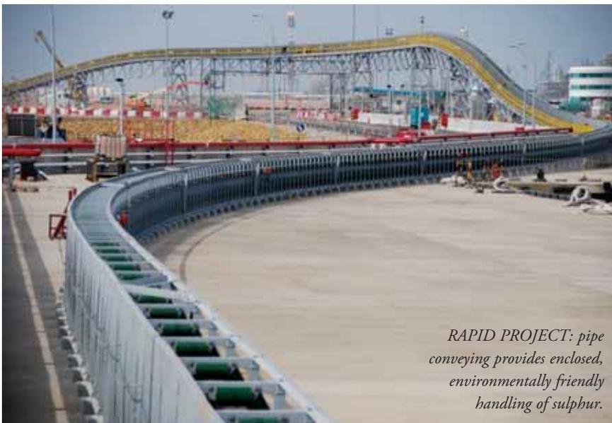
*RAPID PROJECT: pipe conveying provides enclosed, environmentally friendly handling of sulphur.*
