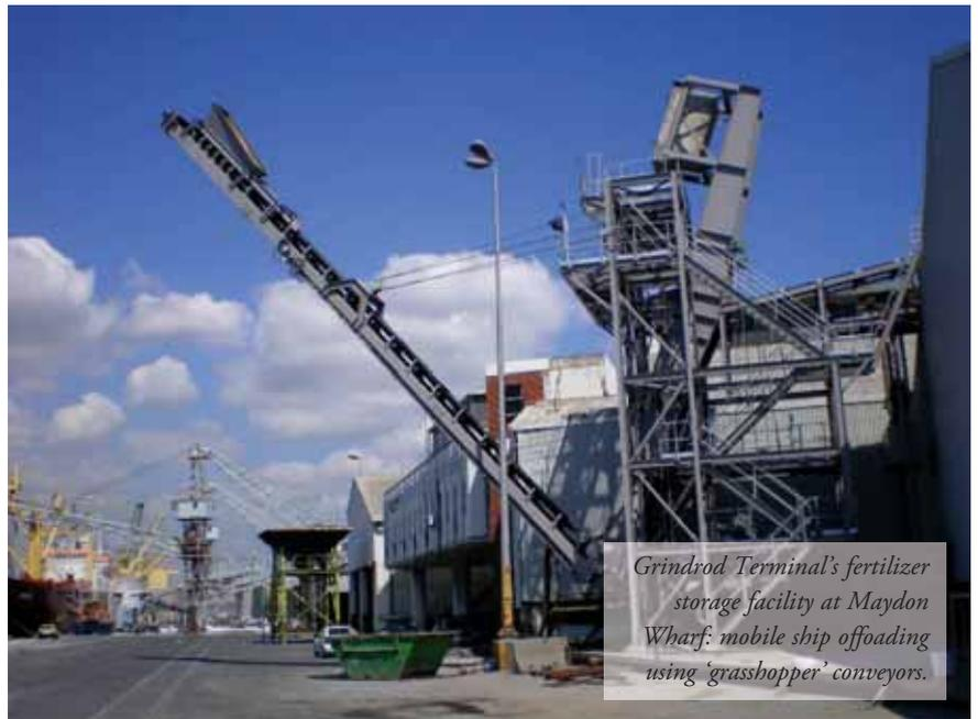
*Grindrod Terminal's fertilizer storage facility at Maydon Wharf: mobile ship offloading using 'grasshopper' conveyors.*
