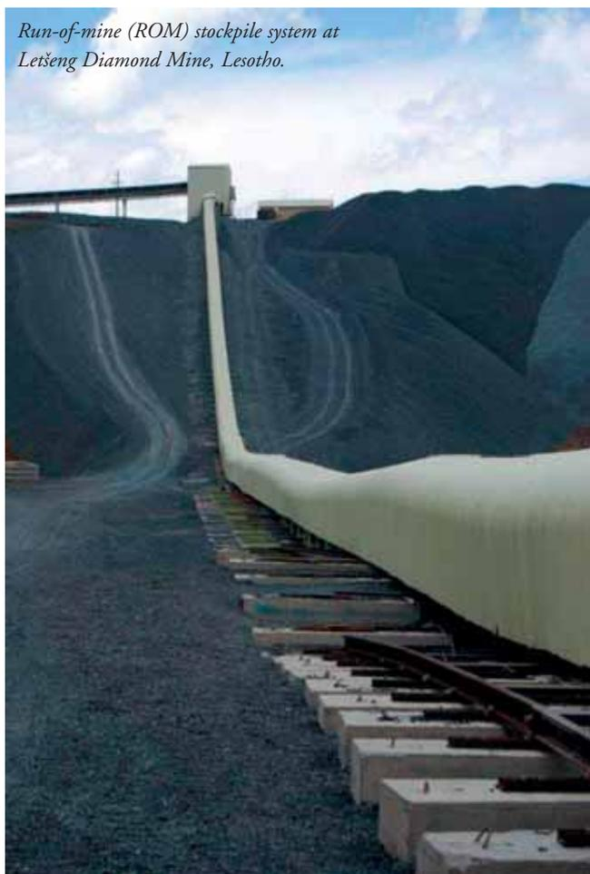
required, considering a number of parameters including partitioning to eliminate material contamination, material size, shape of the stockpiles, terrain limitations, stacking methodology, stockyard layout and equipment selection.
