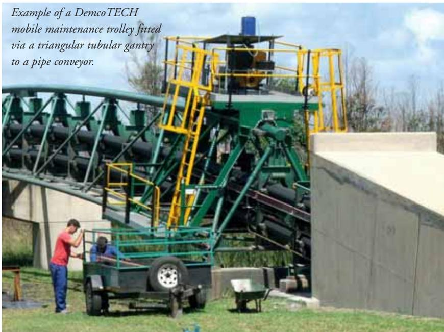
site. The trolleys are self-propelled by an on-board generator and include hydraulically driven travel mechanisms for a high level of control. The trolley designs include a number of safety features such as fully enclosed access facilities, emergency brake systems and heavy duty traction control.
